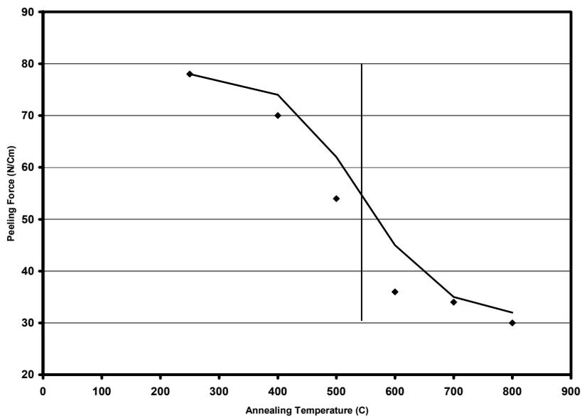
Figure3: Variation of peeling force versus annealing temperature.
