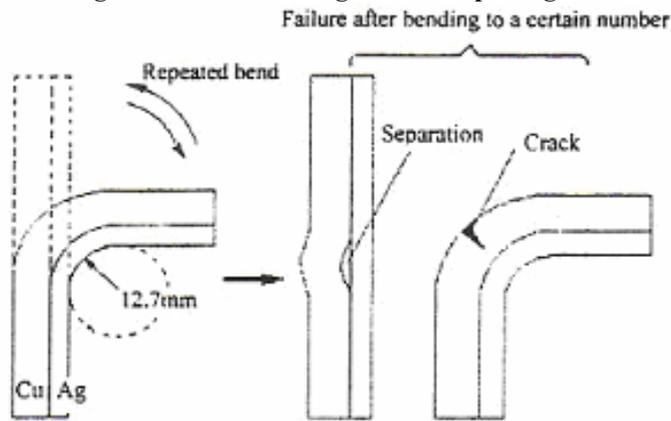
Figure2: Schematic diagram of the bending test.
