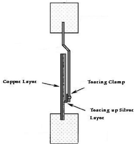
Figure1: Schematic diagram of the peeling test.
